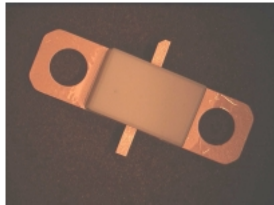
Figure 4. A 10 Watt discrete PHEMT transistor in a bolt down non-hermetic package.
